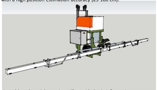
For chemical weed control in wheat, aerial units will generate weed infestation maps. This information will be provided to a fleet of autonomous mediumsize sprayers. These vehicles will be equipped with GPS, sensors, control systems and leading edge injection systems and solenoid valves to spray diferentially various herbicides in different field areas.
