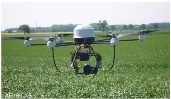
The aerial units are based on quadrotors (AirRobot AR100X6) with a weight of 1.6 kg and a payload of 680 g. They are capable to carry and control small cameras that will monitor fields in order to acquire relevant data with a high position estimation accuracy (25-100 cm).
