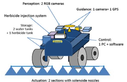
For chemical weed control in wheat, aerial units will generate weed infestation maps. This information will be provided to a fleet of autonomous medium-size sprayers. These vehicles will be equipped with GPS, sensors, control systems and leading edge injection systems and solenoid valves to spray differentially various herbicides in different field areas.
