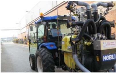
working width of the machine is 3 m covering 4 crop rows spaced 75 cm. The systems for the LPG feeding, the ignition of the burners and all the sensors were implemented on this machine. In October 2012 a technical meeting took place in Pisa in order to verify the proper functioning of the implement. Blubotics, in collaboration with the UP, have installed and connected the PLC and, finally, successfully tested the low level actuation system and devices system.
