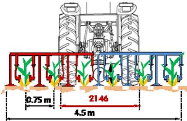
First prototype of precision hoe for mechanical and thermal weed control
